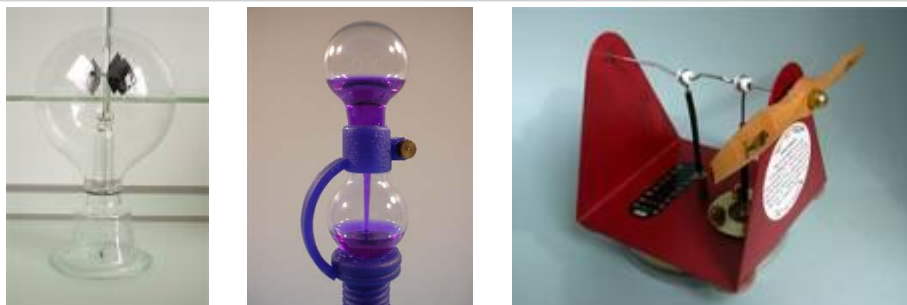
Fig. 25. Simple experiments to enrich the discussion on energy transformations - heat into mechanical work: Crookes "wind-mill"; "love meter"; Stirling's engine
